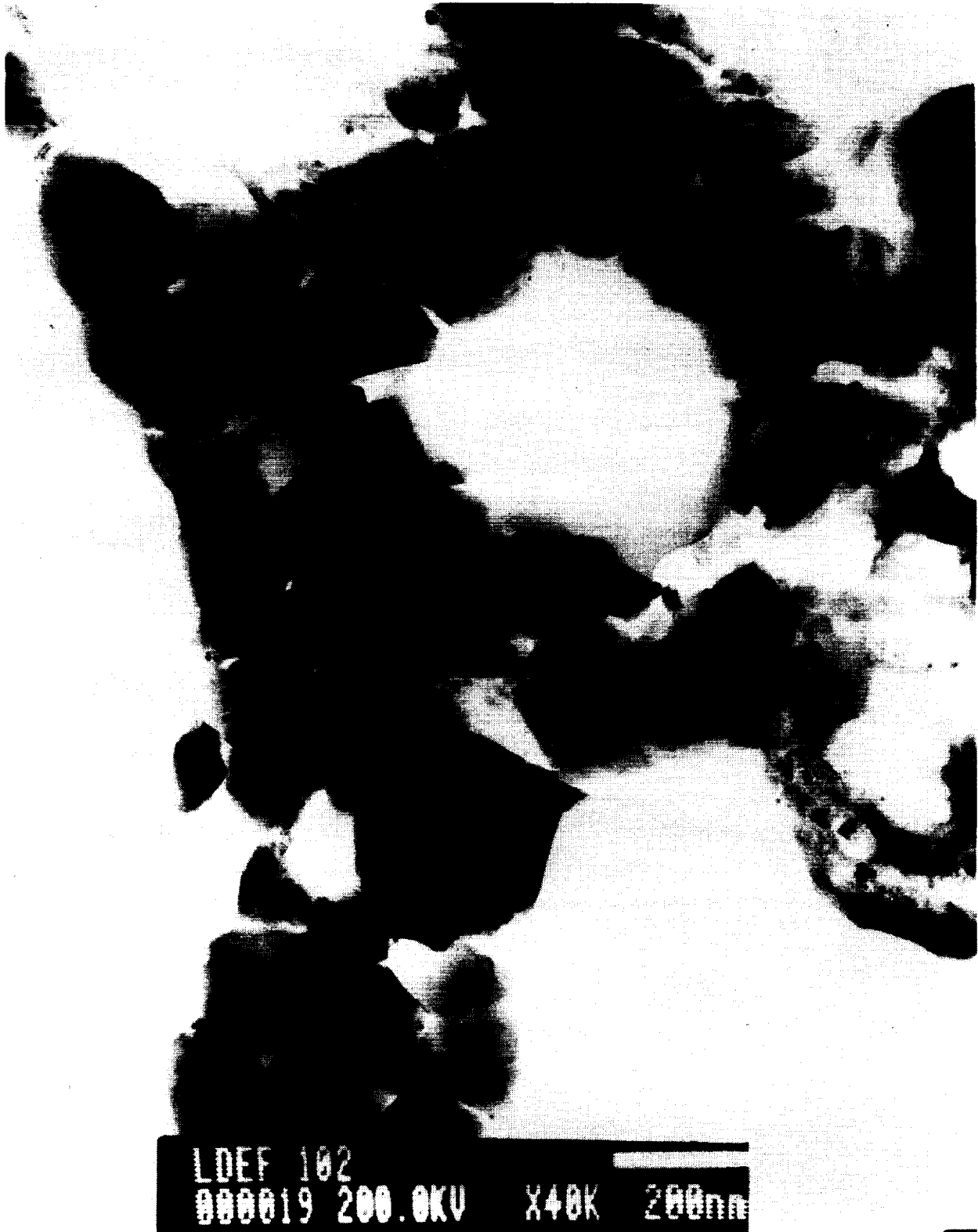
Figure 5. A TEM image of a microtomed residue grain from impact 102. Pyroxene crystals in the field of view have been recrystallized, as indicated by 120° grain intersections.
