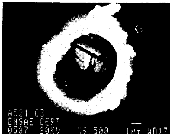
Figure a: Oblique impact (6.6 x 5.4 \mu\text{m} ) on 99% pure Al experiment surface.
