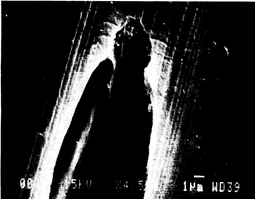
Figure 5. Undercut cavity beneath a narrow crack in the aluminized coating after removal of the aluminized coating.
