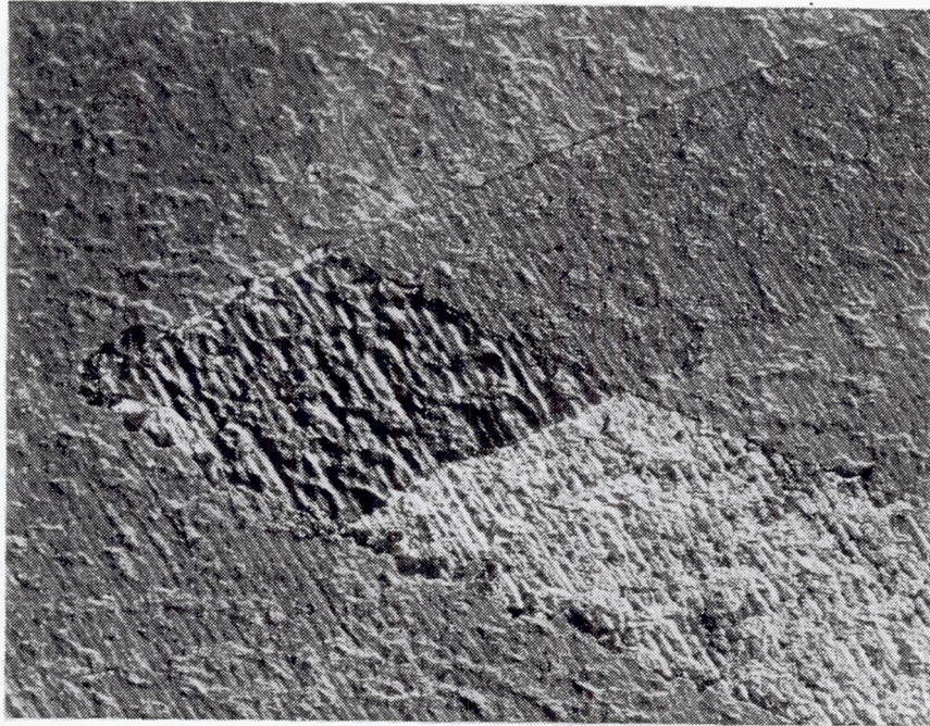
Figure 85 Photograph of Junction Area of Sensor RFS-S1 After Two Cycles to 1144K
