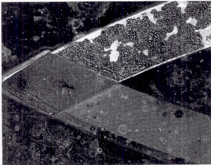
Figure 80 Photograph of Junction Area of Sensor IIE-C2 After Four Cycles to 1144K
