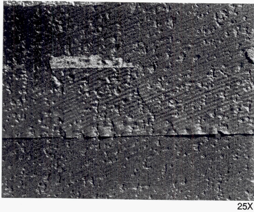
Figure 92 Photograph of Rhodium Leg of Sensor RFS-S2 After One Cycle to 1144K
