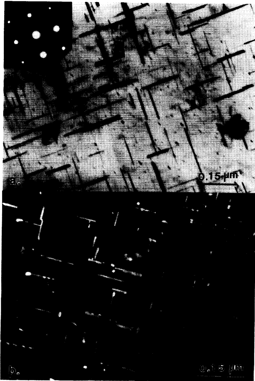
Figure 11. Precipitates in Al_{11}M/SiC_p , a) sample aged at 250C 2 hours, b) sample aged at 200C, 3 hours, diffraction pattern shows the reflections of s' and \theta' phase.
