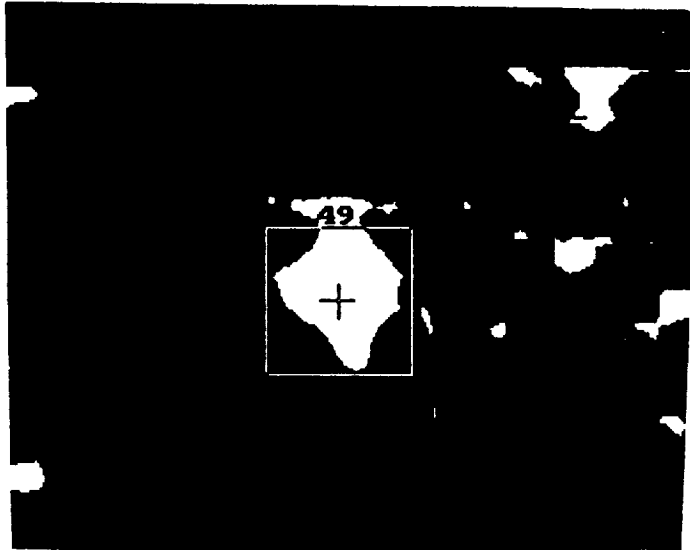
(b) Stitched Specimen # STSI-15: C-Scan Damage Area = 446 mm 2
