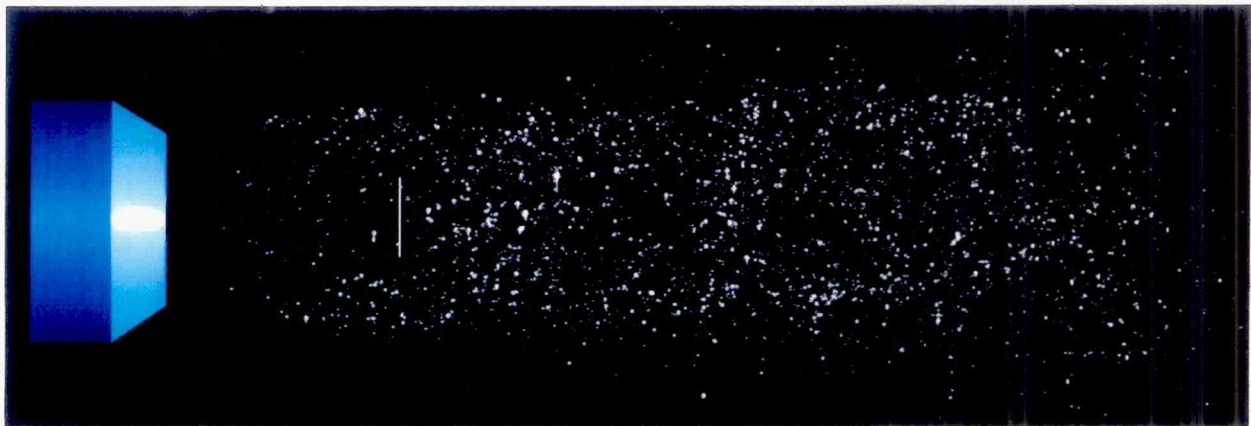
Figure 2.—Raw PIV image from camera. The location of the Mach disk is indicated by the vertical white line.
