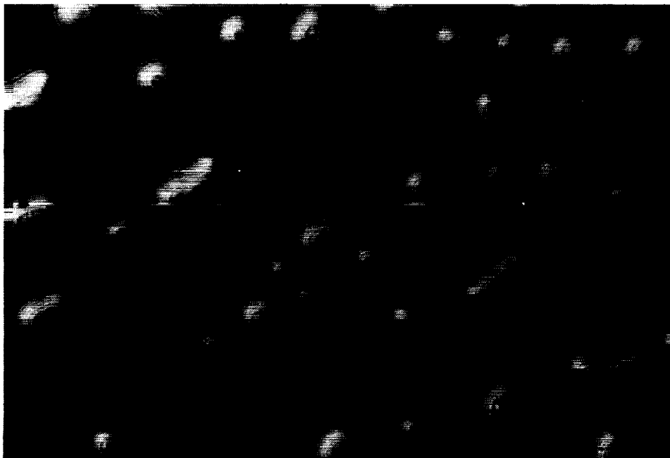
Figure 17a. Optical micrograph of leading-edge ZnS-witness sample (L3-II-7-65-10) after 70-month exposure in LEO. The coating is buckled and annular features are observed at this magnification (168X). (Micrograph courtesy of S. Gyetvay, Aerospace Corporation.)
