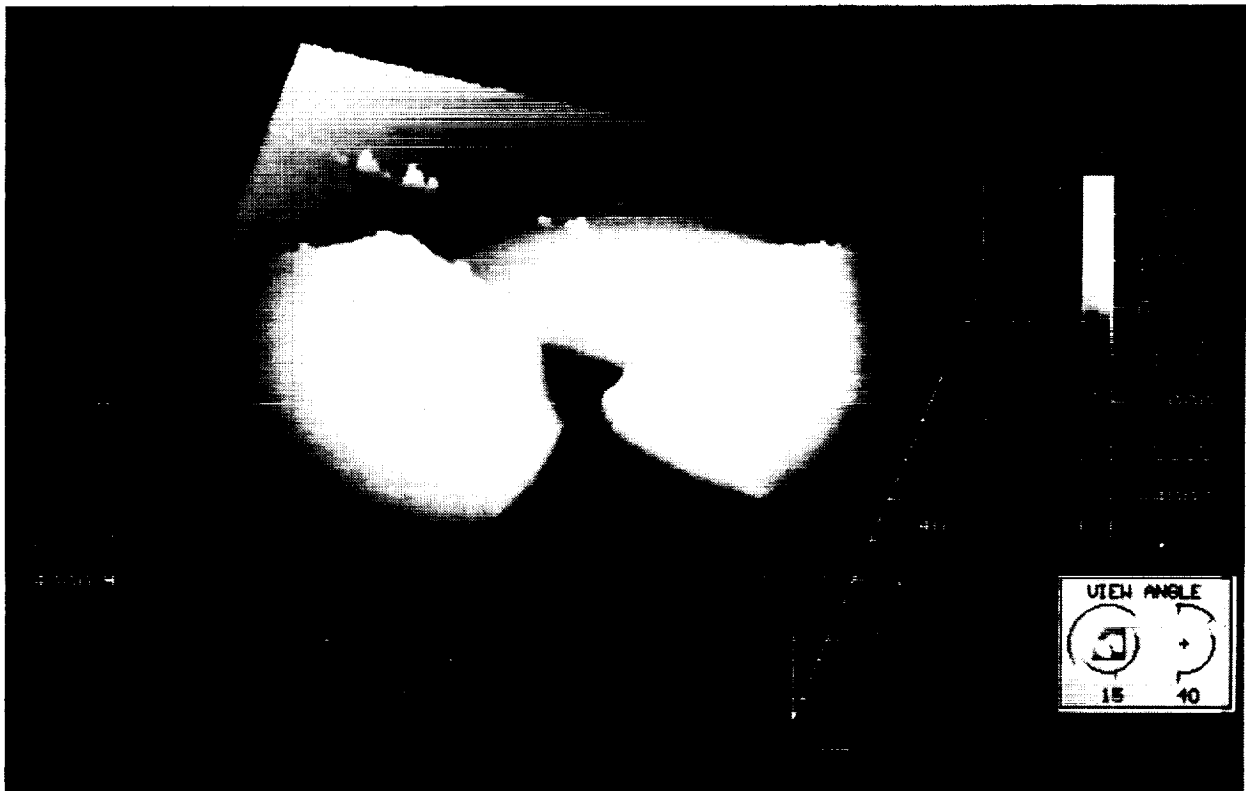
Figure 4b. Atomic force micrograph of impact site in Figure 4a showing the impact crater and film delamination surrounding the crater.
