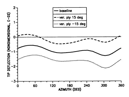
Figure 10.6: Effect of vertical wall ply angle on blade tip response; torsion mode ( $\mu = 0.30$ ).
