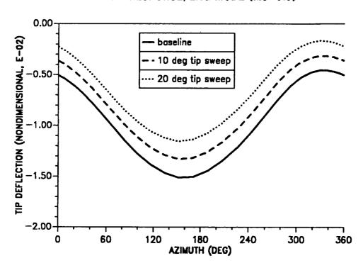
Figure 10.7: Effect of tip sweep angle on blade tip response; lag mode  $(\mu = 0.30)$ .
