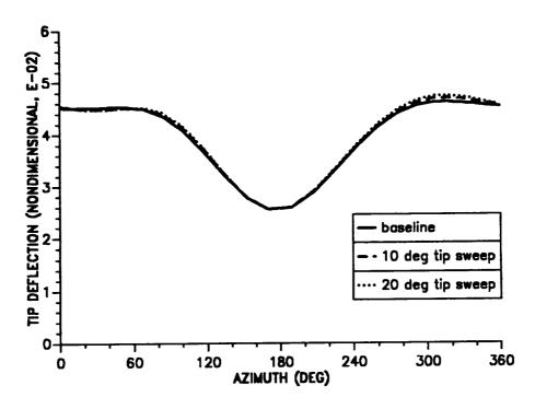
Figure 10.8: Effect of tip sweep angle on blade tip response; flap mode  $(\mu = 0.30)$ .
