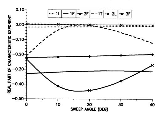
Figure 10.37: Effect of tip sweep angle on blade stability for the first six modes, modified torsional frequency ( $\mu = 0.30$ ).
