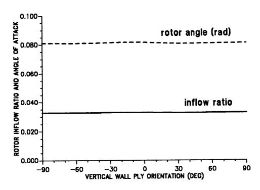
Figure 10.16: Effect of vertical wall ply angle on trim variables; inflow and rotor angle of attack ( $\mu = 0.30$ ).
