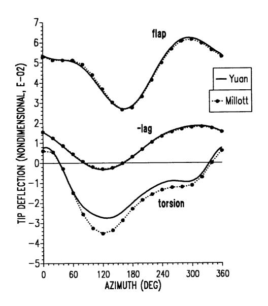
Figure 8.14: Blade tip response for stiff-in-plane isotropic blade ( $\mu = 0.30$ ).
