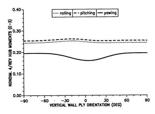
Figure 10.24: Effect of vertical wall ply angle on 4/rev hub moments  $(\mu = 0.30)$ .
