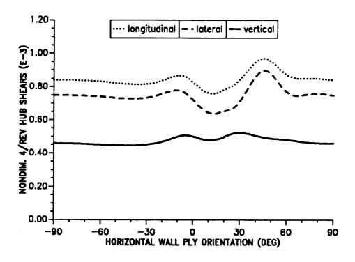
Figure 10.21: Effect of horizontal wall ply angle on 4/rev hub shears  $(\mu = 0.30)$ .
