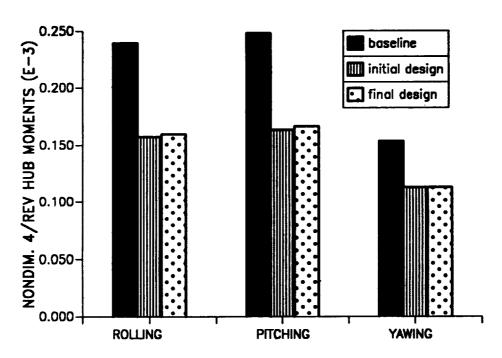
Figure 11.6: The 4/rev hub moments corresponding to second blade configuration (soft-in-plane) and first objective function ( $\mu = 0.30$ ).
