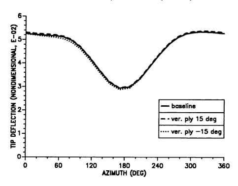
Figure 10.5: Effect of vertical wall ply angle on blade tip response; flap mode  $(\mu = 0.30)$ .
