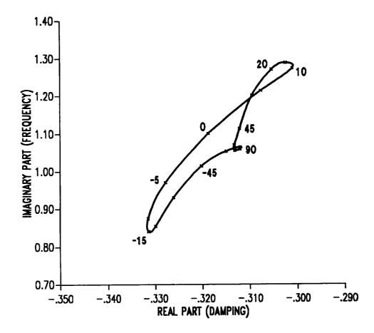
Figure 9.19: Root locus of first flap mode eigenvalues as a function of ply angle in horizontal wall for single-cell composite blade in hover.
