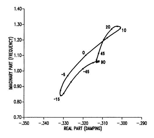
Figure 9.20: Root locus of first torsion mode eigenvalues as a function of ply angle in horizontal wall for single-cell composite blade in hover.
