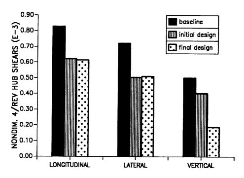
Figure 11.3: The 4/rev hub shears corresponding to first blade configuration (soft-in-plane) and second objective function ( $\mu = 0.30$ ).
