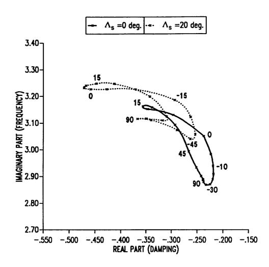
Figure 9.29: Root locus of second flap mode eigenvalues as a function of ply angle in horizontal wall for two-cell composite blade in hover.
