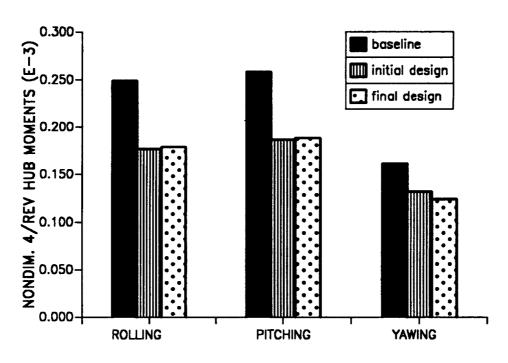
Figure 11.2: The 4/rev hub moments corresponding to first blade configuration (soft-in-plane) and first objective function ( $\mu = 0.30$ ).
