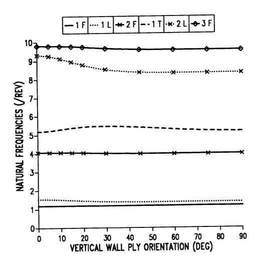
Figure 9.1: Natural frequencies as a function of ply angle in vertical wall for single-cell composite blade.
