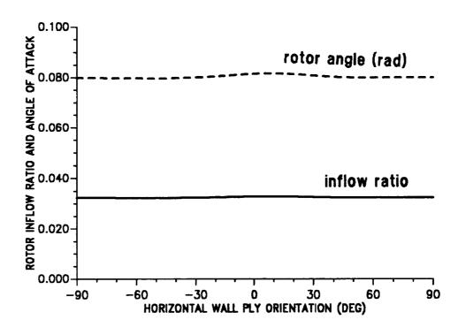
Figure 10.14: Effect of horizontal wall ply angle on trim variables; inflow and rotor angle of attack ( $\mu = 0.30$ ).
