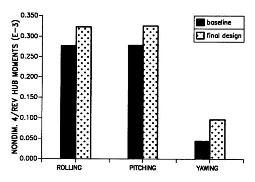
Figure 11.12: The 4/rev hub moments corresponding to third blade configuration (stiff-in-plane) and second objective function  $(\mu = 0.30)$ .
