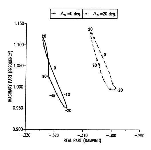
Figure 9.27: Root locus of first flap mode eigenvalues as a function of ply angle in horizontal wall for two-cell composite blade in hover.
