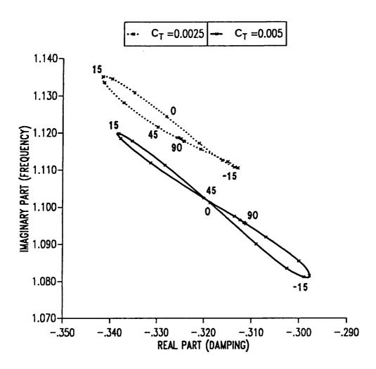
Figure 9.16: Root locus of first flap mode eigenvalues as a function of ply angle in vertical wall for single-cell composite blade in hover.
