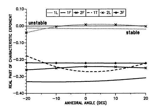
Figure 10.35: Effect of tip anhedral angle on blade stability for the first six modes ( $\mu = 0.30$ ).
