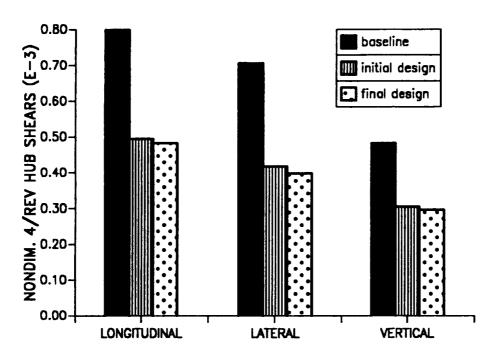
Figure 11.5: The 4/rev hub shears corresponding to second blade configuration (soft-in-plane) and first objective function ( $\mu = 0.30$ ).
