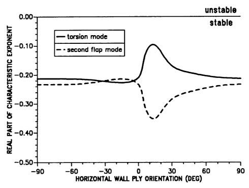
Figure 10.36: Effect of horizontal wall ply angle on stability of first torsion and second flap modes, modified torsional frequency  $(\mu = 0.30)$ .
