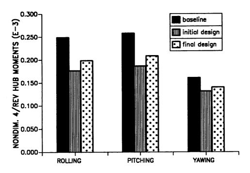
Figure 11.4: The 4/rev hub moments corresponding to first blade configuration (soft-in-plane) and second objective function ( $\mu = 0.30$ ).
