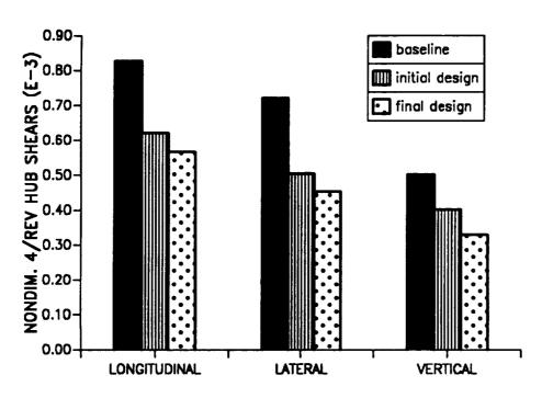
Figure 11.1: The 4/rev hub shears corresponding to first blade configuration (soft-in-plane) and first objective function ( $\mu = 0.30$ ).
