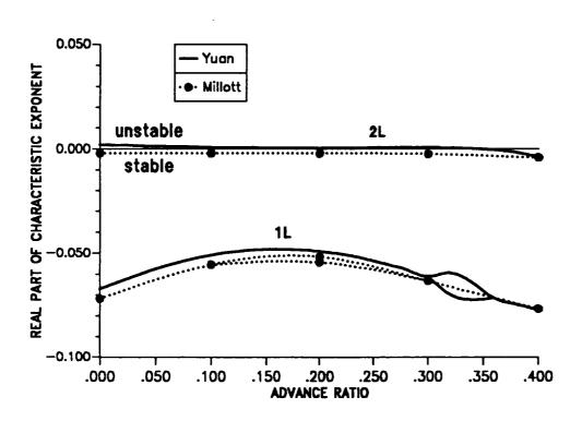
Figure 8.18: Blade damping for stiff-in-plane isotropic blade in forward flight; first and second lag modes.
