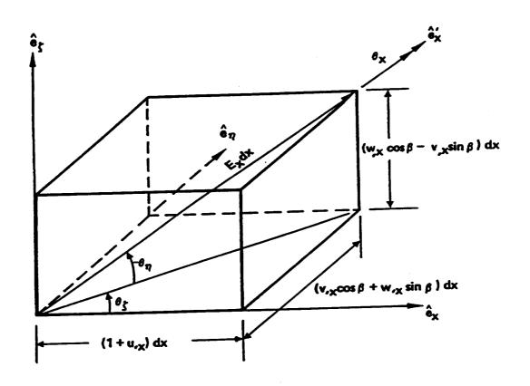
Figure 3.1: Deformation sequence and Euler angles
