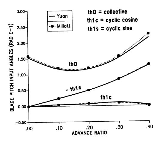
Figure 8.11: Trim variables for stiff-in-plane isotropic blade in forward flight; pitch setting.
