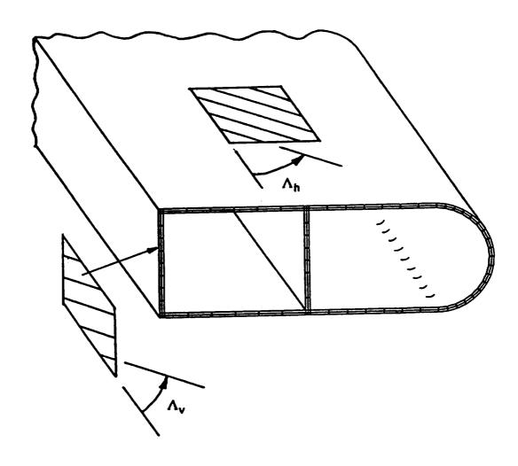
Figure 7.1: Finite element model for two-cell composite cross section
