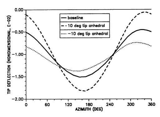
Figure 10.10: Effect of tip anhedral angle on blade tip response; lag mode  $(\mu = 0.30)$ .
