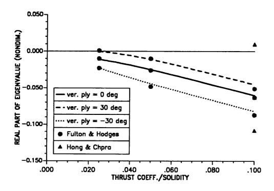
Figure 8.8: Real part of hover eigenvalues for single-cell composite blade as a function of (thrust coefficient/solidity).
