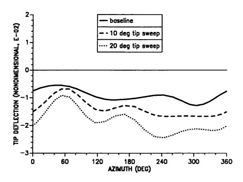
Figure 10.9: Effect of tip sweep angle on blade tip response; torsion mode  $(\mu = 0.30)$ .
