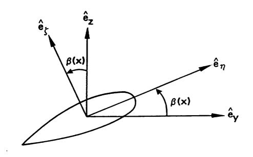
Figure 2.4: Undeformed curvilinear coordinate system
