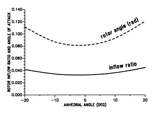
Figure 10.20: Effect of tip anhedral angle on trim variables; inflow and rotor angle of attack ( $\mu = 0.30$ ).
