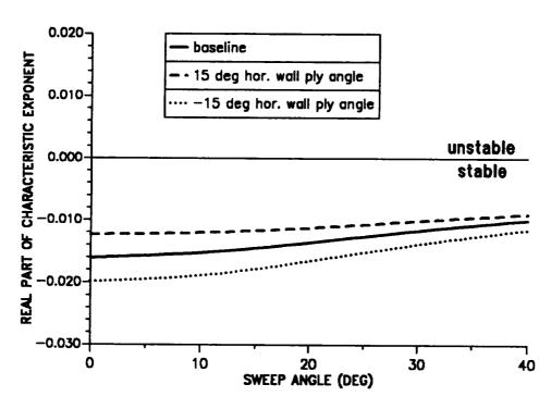
Figure 10.44: Real part of characteristic exponent of blade first lag mode as a function of tip sweep angle, combined effect with ply orientation ( $\mu = 0.30$ ).
