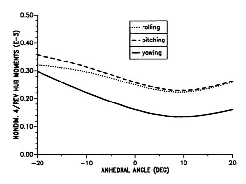
Figure 10.28: Effect of tip anhedral angle on 4/rev hub moments ( $\mu = 0.30$ ).
