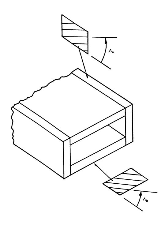
Figure 8.7: Single-cell composite rectangular box beam
