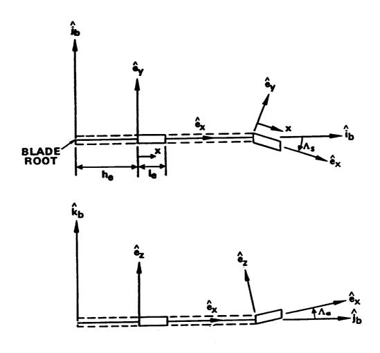
Figure 2.3: Undeformed element coordinate system
