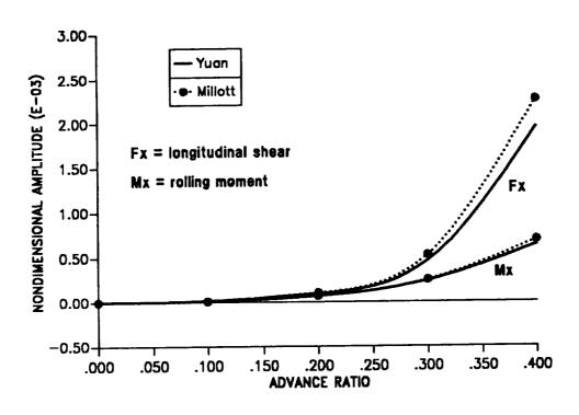
Figure 8.21: The 4/rev hub loads for soft-in-plane isotropic blade in forward flight; logitudinal shear and rolling moment.
