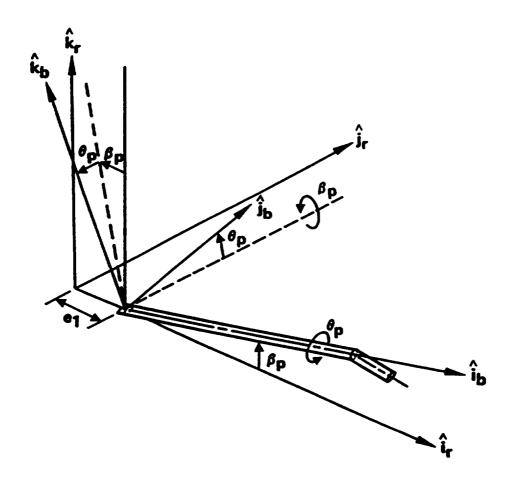
Figure 2.2: Preconed, pitched, blade-fixed coordinate system
