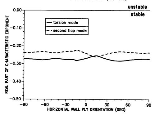
Figure 10.31: Effect of horizontal wall ply angle on blade stability; first torsion and second flap modes ( $\mu = 0.30$ ).
