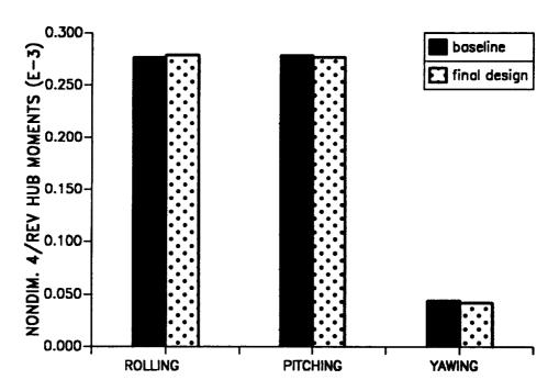
Figure 11.10: The 4/rev hub moments corresponding to third blade configuration (stiff-in-plane) and first objective function ( $\mu = 0.30$ ).
