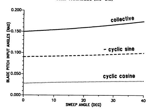
Figure 10.17: Effect of tip sweep angle on trim variables; pitch setting  $(\mu = 0.30)$ .
