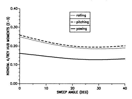
Figure 10.26: Effect of tip sweep angle on 4/rev hub moments ( $\mu = 0.30$ ).
