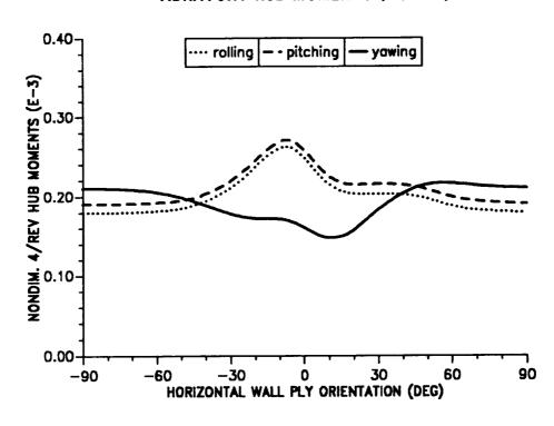
Figure 10.22: Effect of horizontal wall ply angle on 4/rev hub moments  $(\mu = 0.30)$ .
