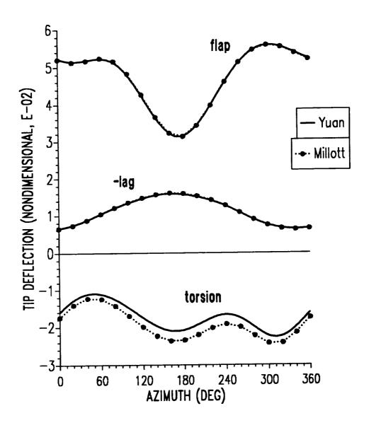
Figure 8.13: Blade tip response for soft-in-plane isotropic blade ( $\mu = 0.30$ ).
