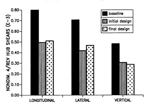
Figure 11.7: The 4/rev hub shears corresponding to second blade configuration (soft-in-plane) and second objective function ( $\mu = 0.30$ ).
