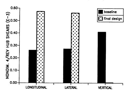
Figure 11.11: The 4/rev hub shears corresponding to third blade configuration (stiff-in-plane) and second objective function ( $\mu = 0.30$ ).
