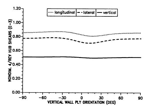
Figure 10.23: Effect of vertical wall ply angle on 4/rev hub shears  $(\mu = 0.30)$ .
