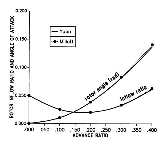
Figure 8.10: Trim variables for soft-in-plane isotropic blade in forward flight; inflow and rotor angle of attack.
