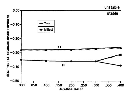
Figure 8.16: Blade damping for soft-in-plane isotropic blade in forward flight; first flap and torsion modes.
