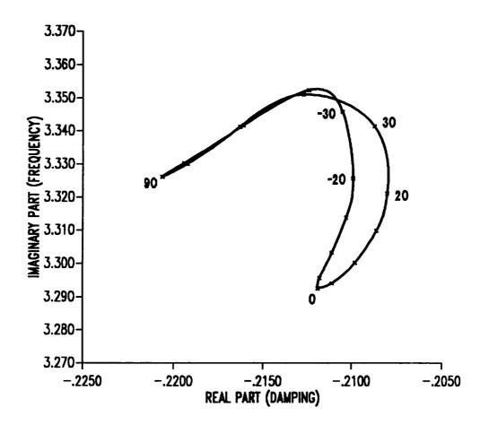
Figure 9.25: Root locus of first torsion mode eigenvalues as a function of ply angle in vertical wall for two-cell composite blade in hover.
