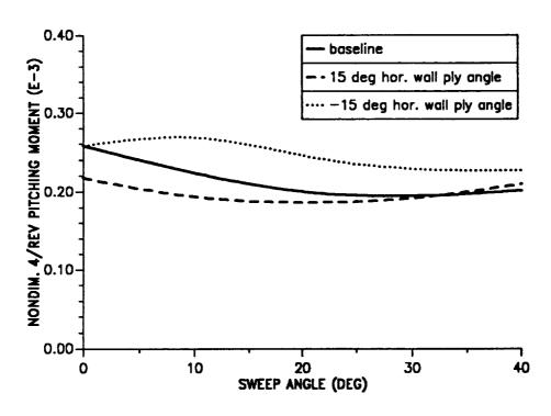
Figure 10.42: The 4/rev hub pitching moment as a function of tip sweep angle, combined effect with ply orientation ( $\mu = 0.30$ ).
