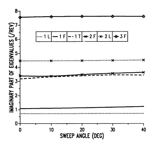
Figure 9.9: Effect of tip sweep on the imaginary part of hover eigenvalues of isotropic blade, modified torsional frequency.
