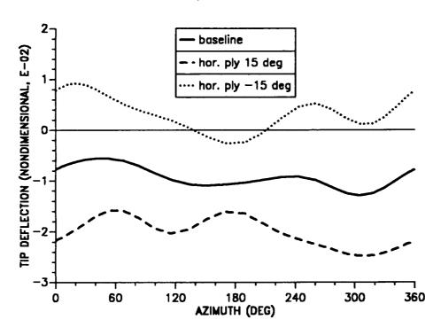
Figure 10.3: Effect of horizontal wall ply angle on blade tip response; torsion mode ( $\mu = 0.30$ ).
