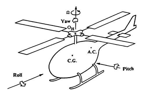
Figure 6.1: Schematic of a four-bladed helicopter
