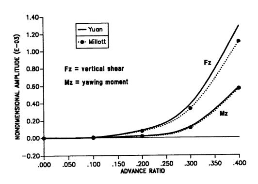
Figure 8.23: The 4/rev hub loads for soft-in-plane isotropic blade in forward flight; vertical shear and yawing moment.
