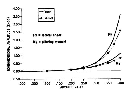
Figure 8.25: The 4/rev hub loads for stiff-in-plane isotropic blade in forward flight; lateral shear and pitching moment.
