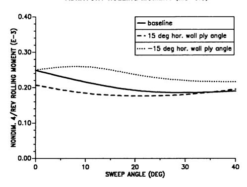
Figure 10.41: The 4/rev hub rolling moment as a function of tip sweep angle, combined effect with ply orientation ( $\mu = 0.30$ ).
