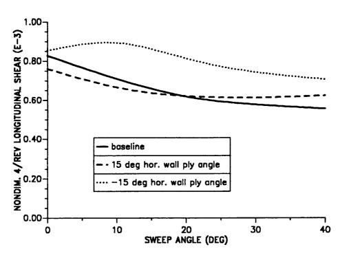
Figure 10.38: The 4/rev longitudinal hub shear as a function of tip sweep angle, combined effect with ply orientation ( $\mu = 0.30$ ).
