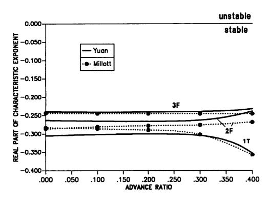
Figure 8.20: Blade damping for stiff-in-plane isotropic blade in forward flight; first torsion, second and third flap modes.
