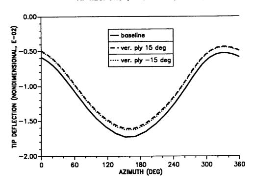
Figure 10.4: Effect of vertical wall ply angle on blade tip response; lag mode  $(\mu = 0.30)$ .
