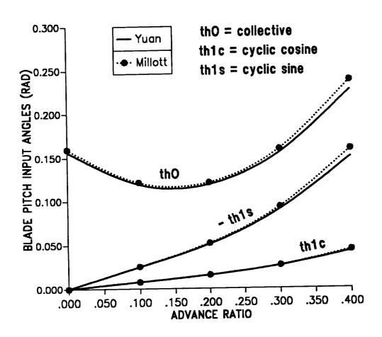
Figure 8.9: Trim variables for soft-in-plane isotropic blade in forward flight; pitch setting.
