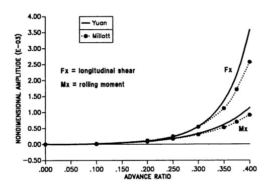
Figure 8.24: The 4/rev hub loads for stiff-in-plane isotropic blade in forward flight; logitudinal shear and rolling moment.
