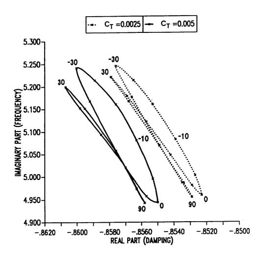
Figure 9.17: Root locus of first torsion mode eigenvalues as a function of ply angle in vertical wall for single-cell composite blade in hover.
