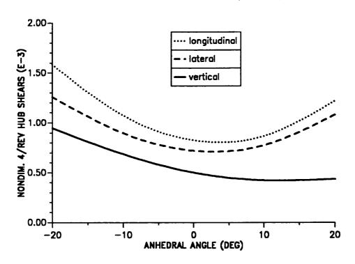
Figure 10.27: Effect of tip anhedral angle on 4/rev hub shears ( $\mu = 0.30$ ).
