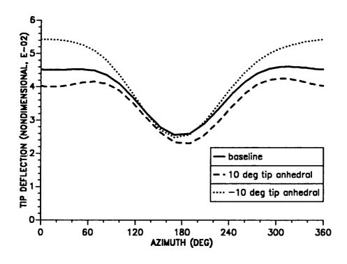
Figure 10.11: Effect of tip anhedral angle on blade tip response; flap mode  $(\mu = 0.30)$ .
