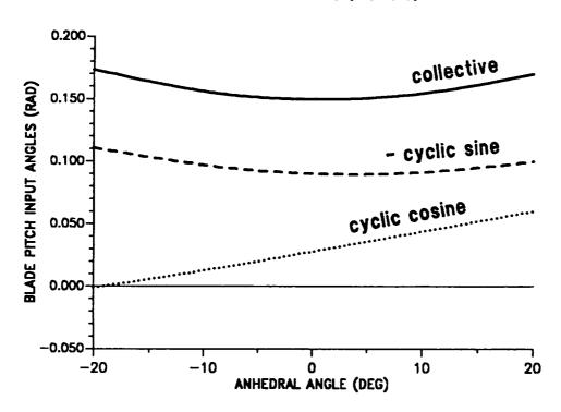
Figure 10.19: Effect of tip anhedral angle on trim variables; pitch setting  $(\mu = 0.30)$ .
