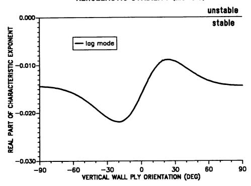
Figure 10.32: Effect of vertical wall ply angle on blade stability; first lag mode ( $\mu = 0.30$ ).
