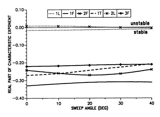
Figure 10.34: Effect of tip sweep angle on blade stability for the first six modes ( $\mu = 0.30$ ).
