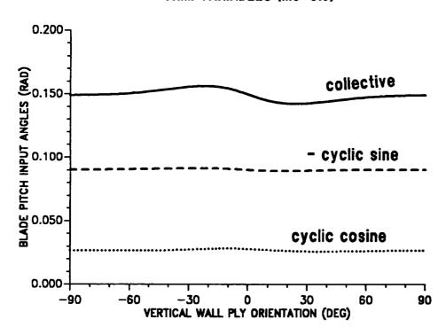
Figure 10.15: Effect of vertical wall ply angle on trim variables; pitch setting  $(\mu = 0.30)$ .
