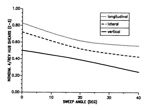
Figure 10.25: Effect of tip sweep angle on 4/rev hub shears ( $\mu = 0.30$ ).
