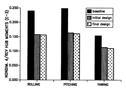
Figure 11.8: The 4/rev hub moments corresponding to second blade configuration (soft-in-plane) and second objective function ( $\mu = 0.30$ ).
