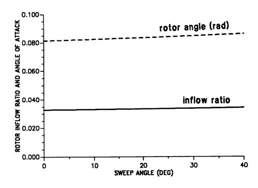
Figure 10.18: Effect of tip sweep angle on trim variables; inflow and rotor angle of attack ( $\mu = 0.30$ ).
