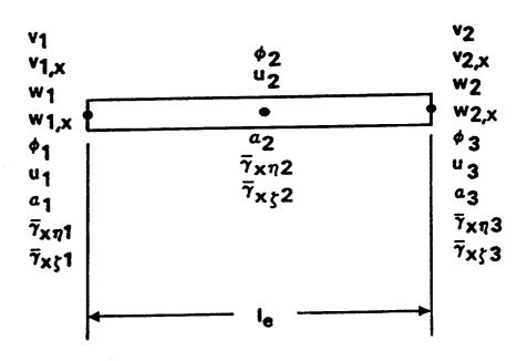
Figure 4.2: Finite element nodal degrees of freedom
