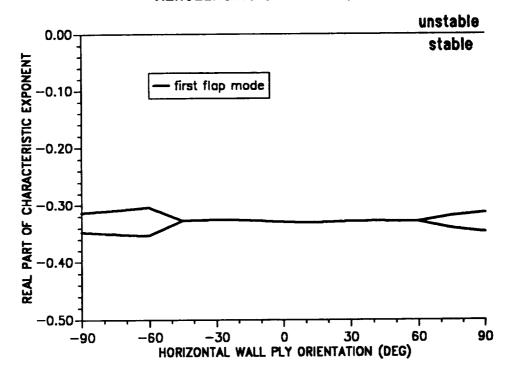
Figure 10.30: Effect of horizontal wall ply angle on blade stability; first flap mode ( $\mu = 0.30$ ).
