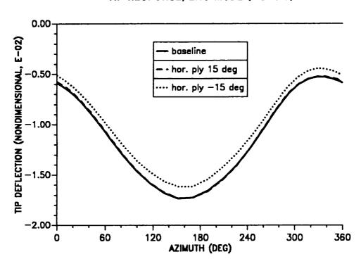
Figure 10.1: Effect of horizontal wall ply angle on blade tip response; lag mode ( $\mu = 0.30$ ).
