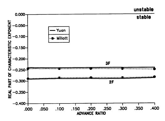
Figure 8.17: Blade damping for soft-in-plane isotropic blade in forward flight; second and third flap modes.
