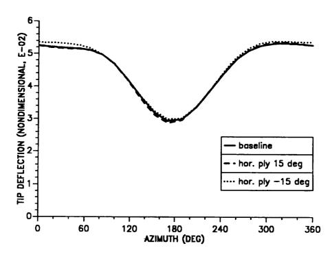
Figure 10.2: Effect of horizontal wall ply angle on blade tip response; flap mode ( $\mu = 0.30$ ).
