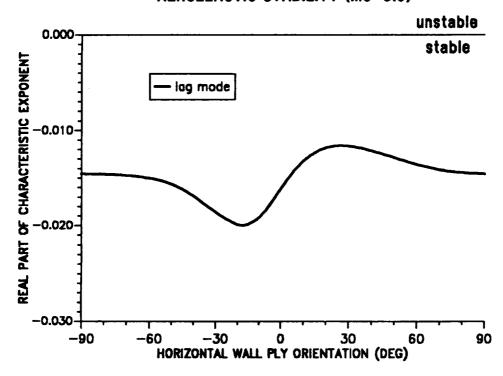
Figure 10.29: Effect of horizontal wall ply angle on blade stability; first lag mode ( $\mu = 0.30$ ).
