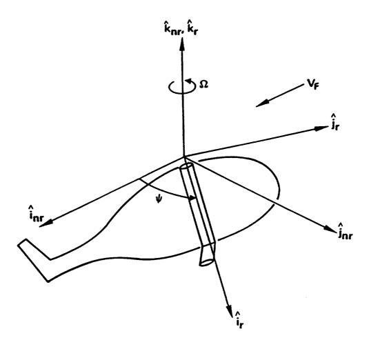
Figure 2.1: Nonrotating, hub-fixed coordinate system and rotating, hub-fixed coordinate system
