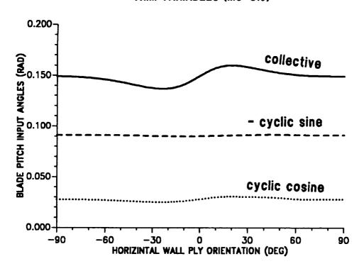
Figure 10.13: Effect of horizontal wall ply angle on trim variables; pitch setting ( $\mu = 0.30$ ).
