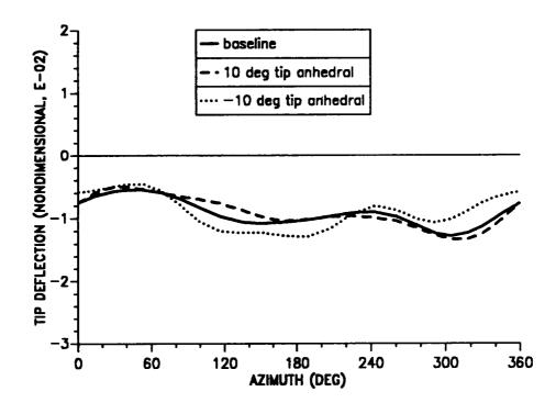
Figure 10.12: Effect of tip anhedral angle on blade tip response; torsion mode ( $\mu = 0.30$ ).
