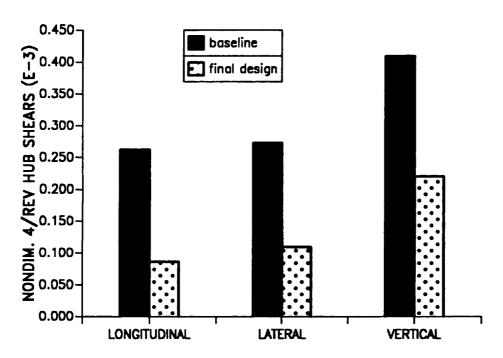
Figure 11.9: The 4/rev hub shears corresponding to third blade configuration (stiff-in-plane) and first objective function ( $\mu = 0.30$ ).
