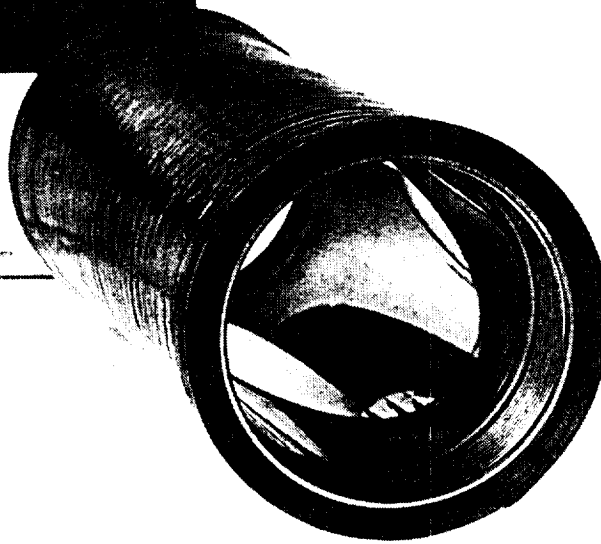
Figure 2. Carbon Epoxy Cylinder with Steel Liner and Thread Inserts
