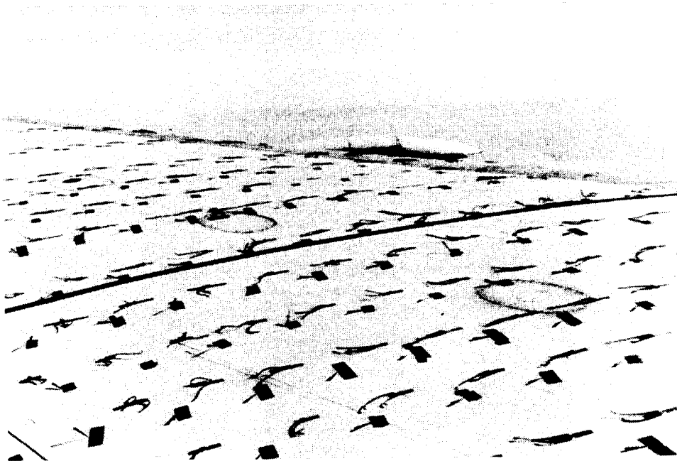
Figure 18. Still photograph showing tufts and cones during reverse-thrust flight at M = 0.55 .
