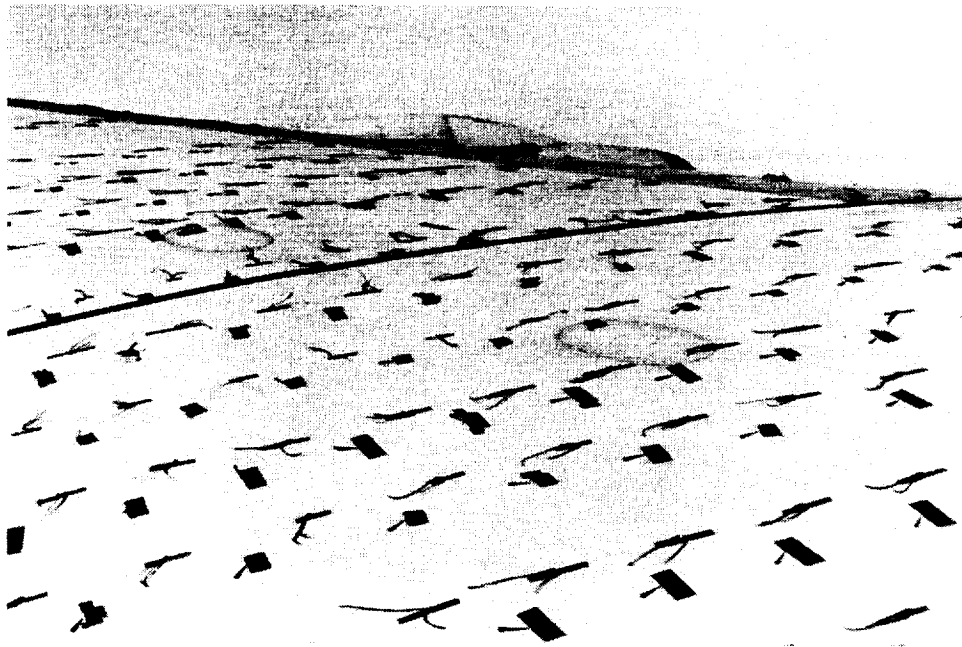
Figure 19. Still photograph showing the tufts and cones during reverse-thrust flight at M = 0.70 .
