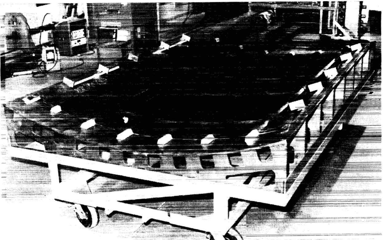
Figure 15: Locating Stringers with IML Cauls
