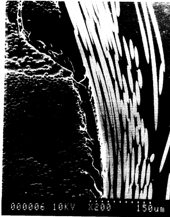
Figure 3. Resin Cavities at Thread
