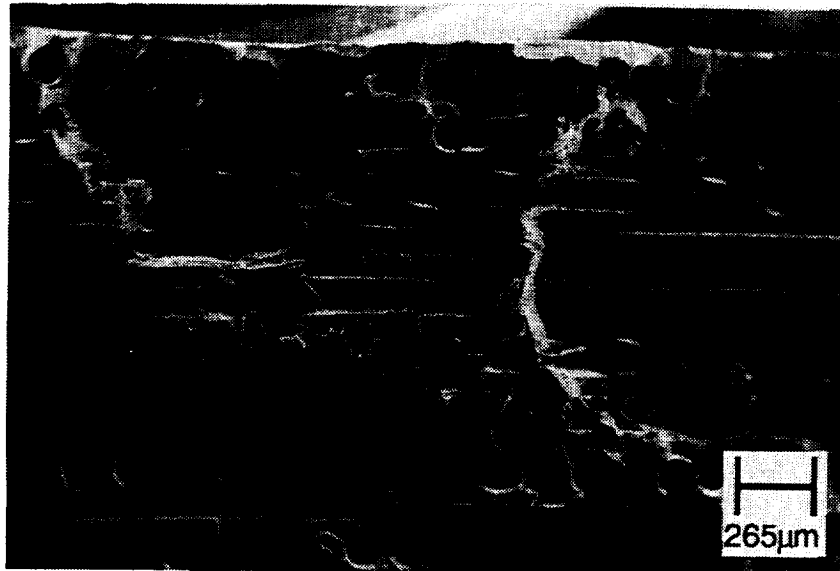
(a) Step-like fracture surface
