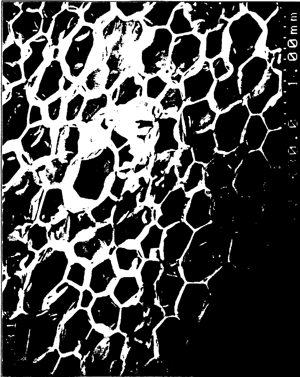
Figure 5. HFC-236ea foam cell structure
