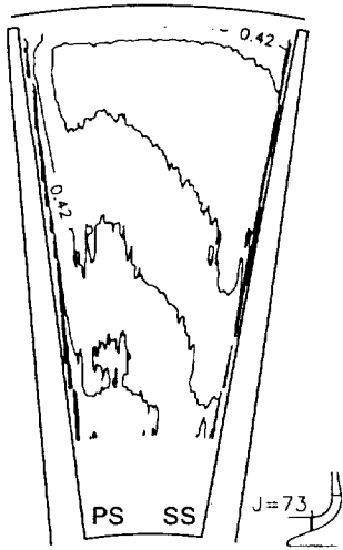
Figure 56 Contour plots of throughflow velocity normalized by impeller tip speed, V_T/U_t , for the design flow condition, \dot{m}_d at station 73 ( m/m_s = 0.030 ).
