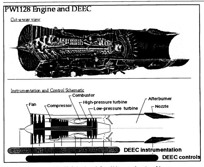
The F-15 is powered by two PW1128 afterburning turbofans which are growth versions of the F100-PW-100 engine. The above schematic shows the engine control effectors and sensor locations. (further details of the PW1128 engine are contained in Myers, et. al., "Digital Electronic Engine Control (DEEC) Flight Evaluation in an F-15 Airplane", NASA CP-2298, Mar 1984).
