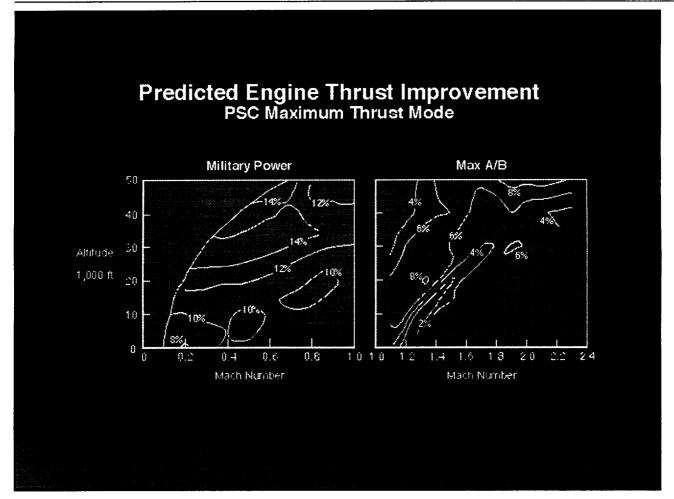
Thrust improvements of up to 14% at military power and up to 8% at maximum power are predicted for the Maximum Thrust Mode.
