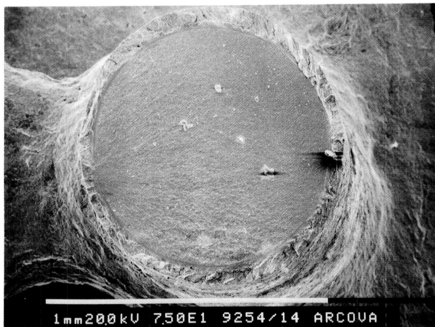
(a) Secondary Electron Image of an Unprocessed Fiber
