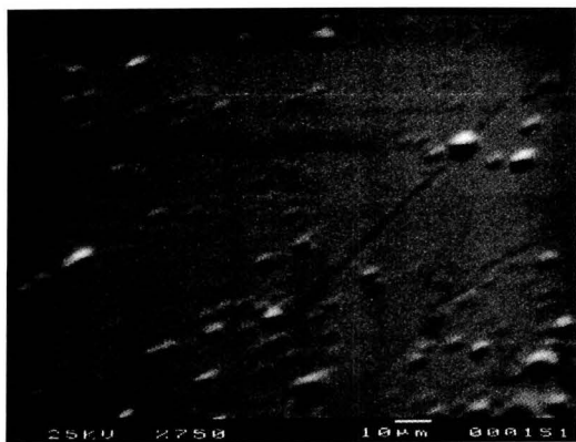
Fig.8. Backscattered SEM picture of a smooth 2122 phase film grown on (110) NdGaO 3 substrate.
