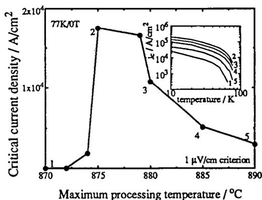
Fig.5 Critical current densities for different maximum processing temperatures at 77K. The inset shows the critical current densities from 10 to 85K.
