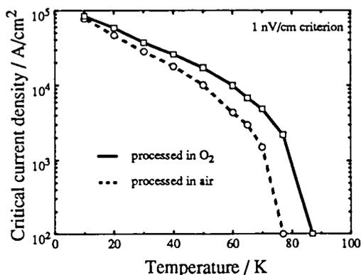
Fig.7 Critical current density for samples processed in air and O<sub>2</sub> from 10 to 85K.
