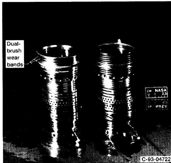
Figure 6.—Compressor discharge seal rotors for labyrinth seal (right) and brush seal (left).
