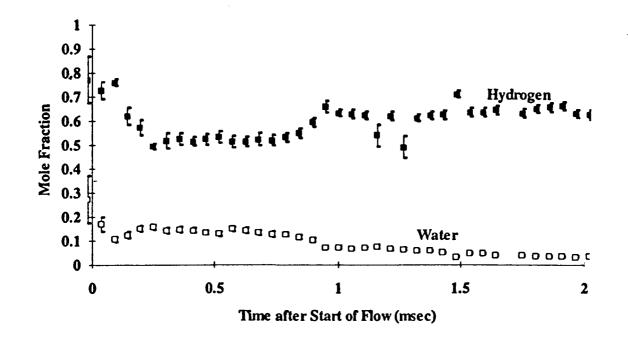
Fig. 3. Mass spectrometer records of hydrogen and water components (stagnation enthalpy = 12.2 MJ kg<sup>-1</sup>, 10 mm from centre line)
