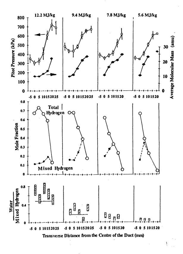
Fig.5 Diffusion of hydrogen and mixing and combustion in wake. (Reaction efficiency: a expt, ------theory.)
