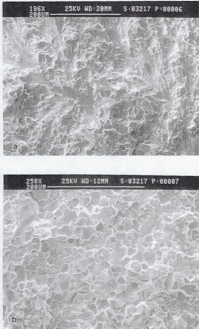
Figure 33. Fracture surfaces of NiAl-300C following tensile testing at room-temperature: (a) as-extruded and (b) after annealing at 1100 K for 2 h followed by furnace cooling.
