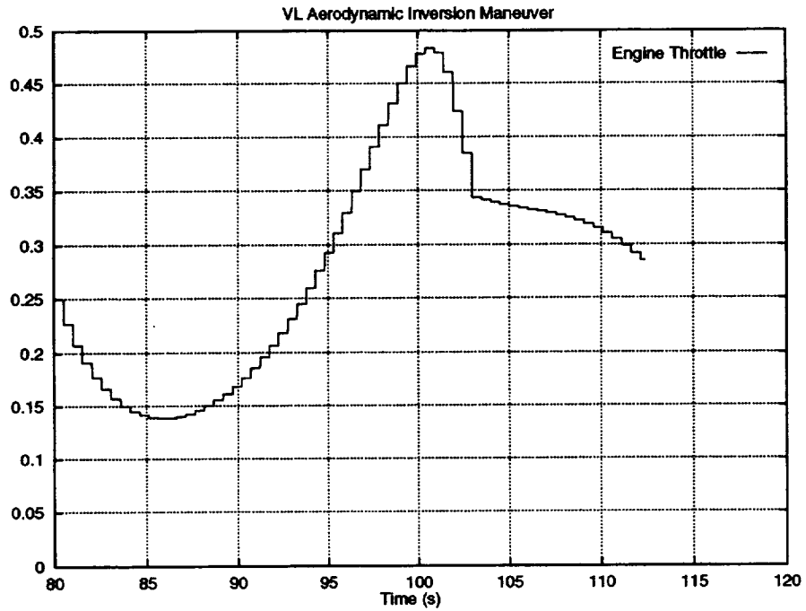
Figure 15. VL aerodynamic inversion maneuver, engine throttle versus time.
