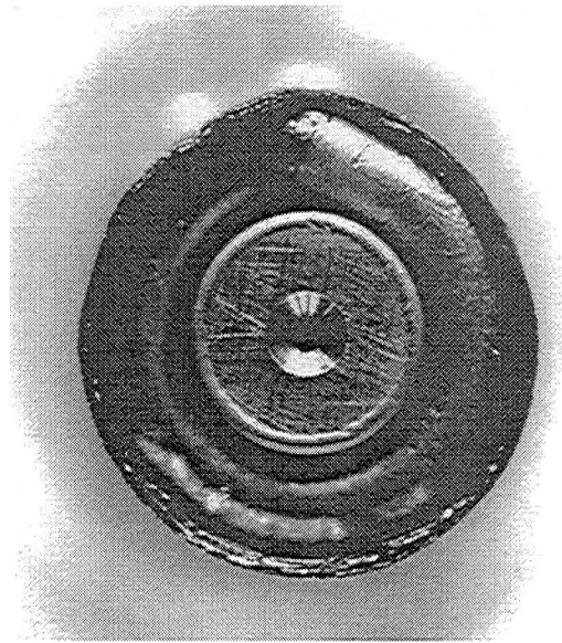
Figure 11a - Pre-test photograph of first wear test discharge cathode
