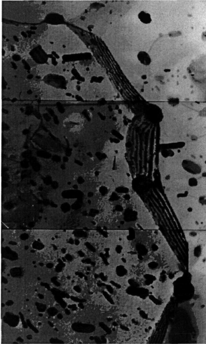
Figure 3. Grain boundary precipitates in alloy K-24 (0.6Cu-0Zr)
