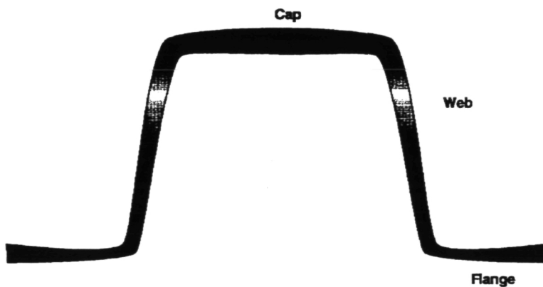
Figure 29. Schematic of SPF beaded web panel cross-section.
