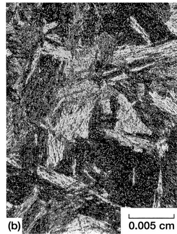
Figure 4.—Photomicrographs of case and core of AISI 9310 test gear. (a) Carburized and hardened case of the CEVM AISI 9310 gear showing high carbon fine grain martensitic structure. (b) Core structure of CEVM AISI 9310 gear showing low carbon refined austenitic grain size.
