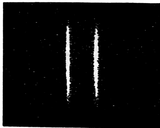
Figure 4. Direct photo of twin flames in a low velocity counterflow field in microgravity.
