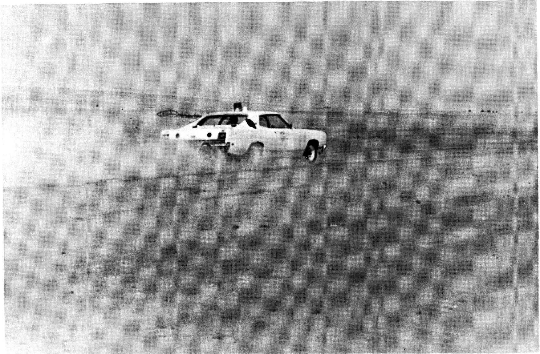
Figure 3.- NASA Diagonal-Braked Vehicle during test run on soil runway at Holland LZ.
