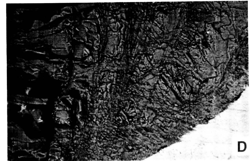
Figure 7. Detailed SEM photographs of highly fractured projectile residue in experiment 3604 at 1.09 km/s. (A) Overview of crater bottom. (B) Partial enlargement illustrating three distinctly different deformation regimes in the form of (1) a relatively coarsely fractured core, (2) intensely comminuted annulus and (3) distinctly plate fragments towards the projectile's rear volume. Note the stunningly sharp contacts between these fragmentation regimes, especially between core and the fine-grained annulus. (C) and (D) Enlarged views of the three fragmentation regimes illuminating details of the highly comminuted lateral portions of the soda-lime glass sphere, characterized by highly localized, two-dimensional zones of severe comminution which we interpret as shear bands. The latter are initially straight and parallel to the central core/annulus contact, but become increasingly curved with lateral distance to parallel the curved crater walls.
