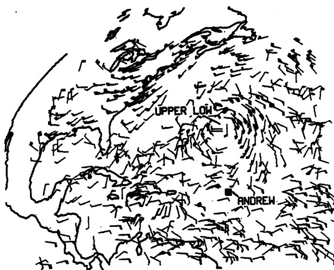
Fig. 1. Typical water vapor wind set coverage.
