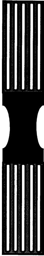
Figure 15 - Proposed integrated-grip dogbone tensile specimen.
