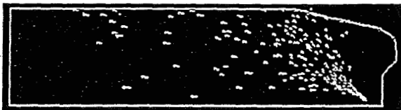
Figure 6. N 2 O 4 spray droplet velocity field.
