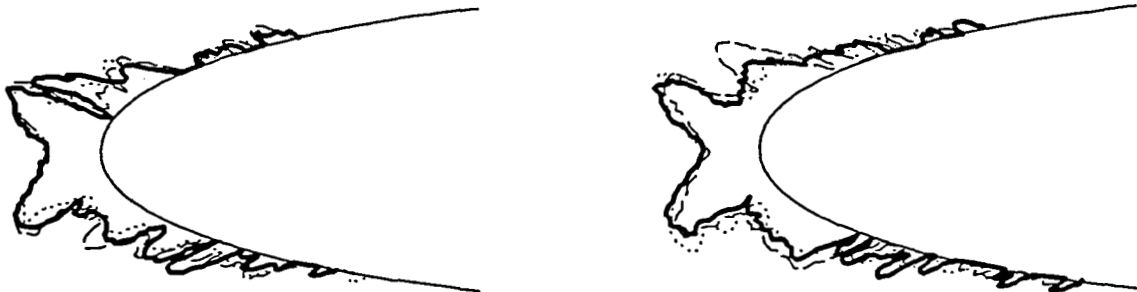
(b) Ice Shapes at 20 cm (8 in) Above Tunnel Centerline.
