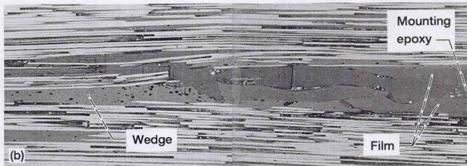
Figure 15.—ENF specimen crack tips after testing 128X. (a) AU-4 fiber, no aging. (b) AU-4 fiber, 1000 hr.
