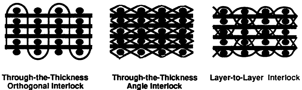
Figure 2. General Schematic of the Three 3-D Weave Types.
