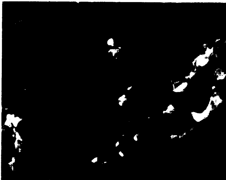
Figure 108. Isolated Microscopic (111) \gamma' Fracture Among Predominantly Matrix Failure; Conditions – PWA 1484 HT 2, Notched LCF, 20°C (68°F), 34.5 MPa (5 ksi) Hydrogen, Magnification 10,000X
