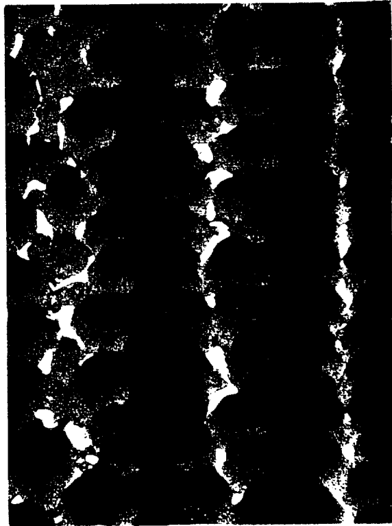
HIP at 1307°C (2385°F)/103 MPa (15 ksi)/4 hr
