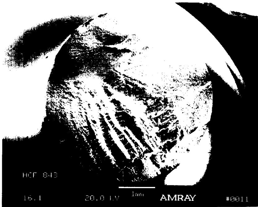
Figure 142. PWA 1484 HT 6 HCF Overall View; Crack Origin Area (At Right) Shows Prominent (111) Fracture; Conditions – PWA 1484 HT 6, 20°C (68°F), 34.5 MPa (5 ksi) Hydrogen, R = -1.0 HCF
