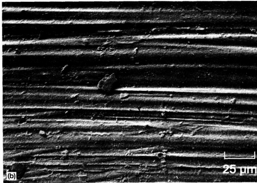
Figure 8.—Photomicrograph of (a) P-100 + Br (b) P-100 + Br (coated w/SiO 2 ) composite after LEO exposure.
