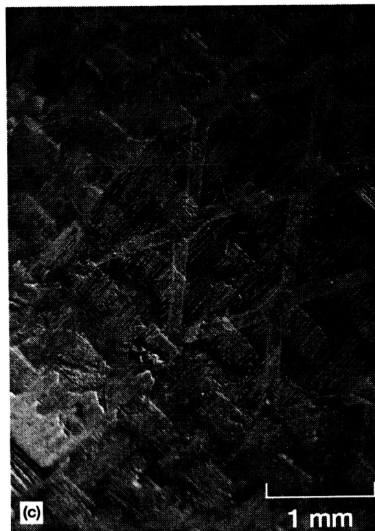
Figure 9.—Photomicrograph of \text{SiO}_2 protected bromine intercalated (a) P-100; (b) P-75; (c) P-55; composite after LEO exposure.
