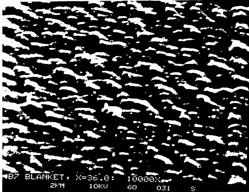
Figure E-17 10000X magnification SEM image of FEP surface 36.0 mm from the edge of blanket B7.
