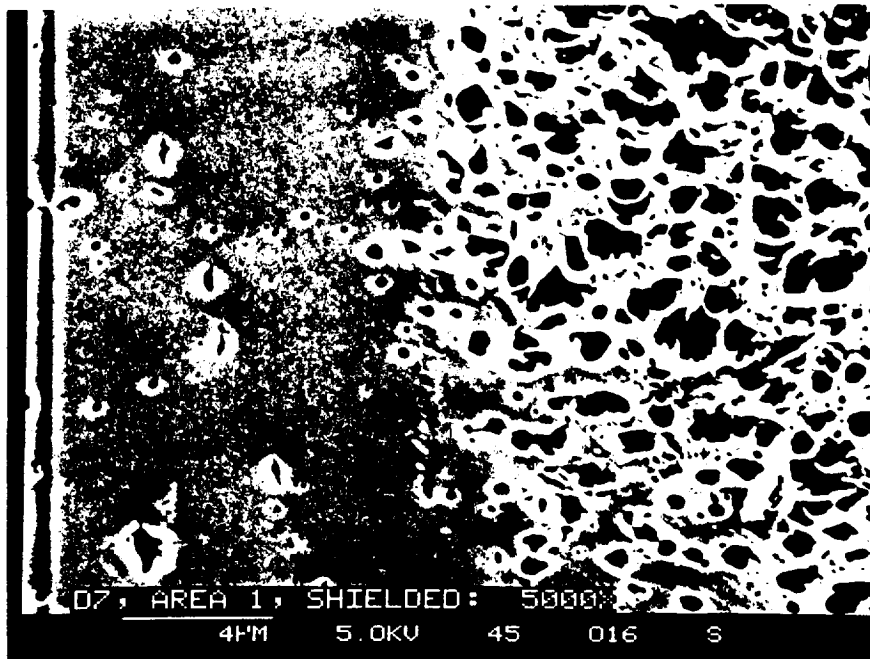
Figure E-46 A 5000X SEM image of the region from D7 shown in the previous figure, with the porous structure of the FEP clearly visible after a low level of atomic oxygen exposure.
