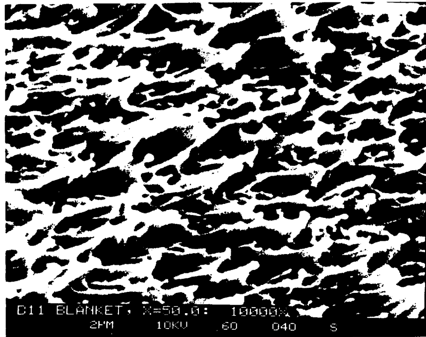
Figure E-12 10000X magnification SEM image of FEP surface 50.0 mm from the edge of blanket D11.
