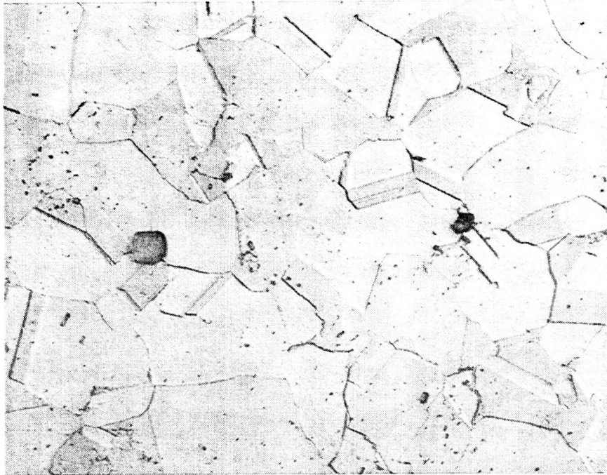
Figure 10a: Optical micrographs showing typical microstructure in the center of a transverse section through the long bolt (etched with Glyceregia). Microhardness measurements indicate Rockwell "C" of 35-36. This corresponds to a tensile strength of 160 ksi.
