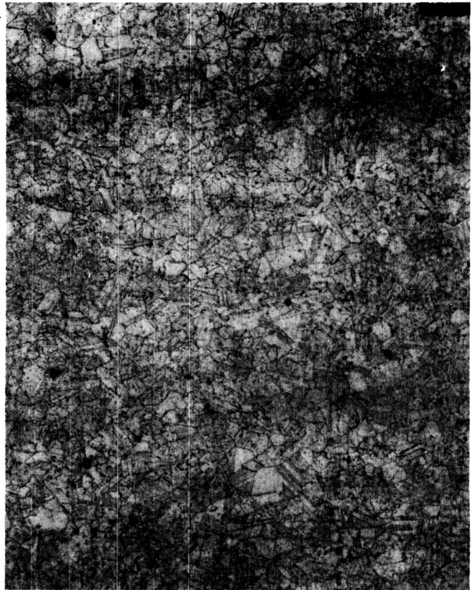
Figure 10. 100X Micrograph of Inconel 718 Used in Qualification Lot under NASA Contract NAS 9-17674.
