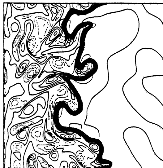
Figure 3. Flame propagation in isotropic turbulence. Contours in the reactants (left of flame) represents vorticity.
