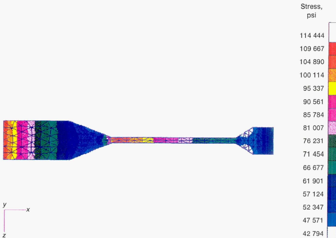
Figure 6.—Fringe plot of von Mises stress for 10th-stage rotating disk of E 3 high-pressure compressor.
