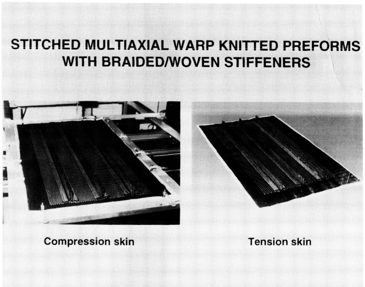
Figure 9. Stitched multiaxial warp knitted preforms with braided/woven stiffeners.
