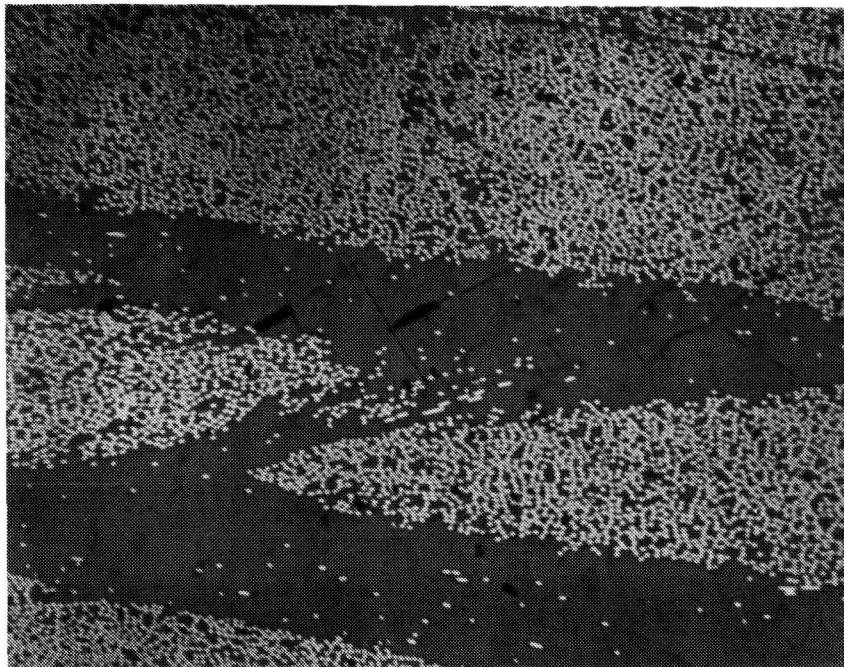
Figure 5 - Matrix Cracking in the LSS Architecture as a Result of Compression Loading
