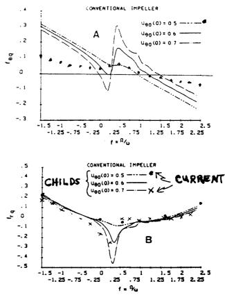
Figure 2. Nomdimensional force coefficients for the conventional impeller (a) tangential-force coefficient, (b) radial-force coefficient
