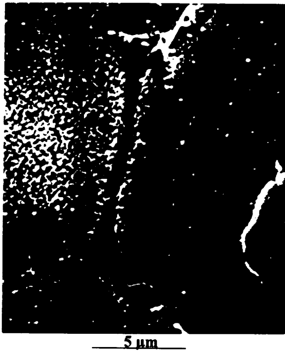
Figure 2.- SEM micrographs showing G.B. with a crack-like shape.
