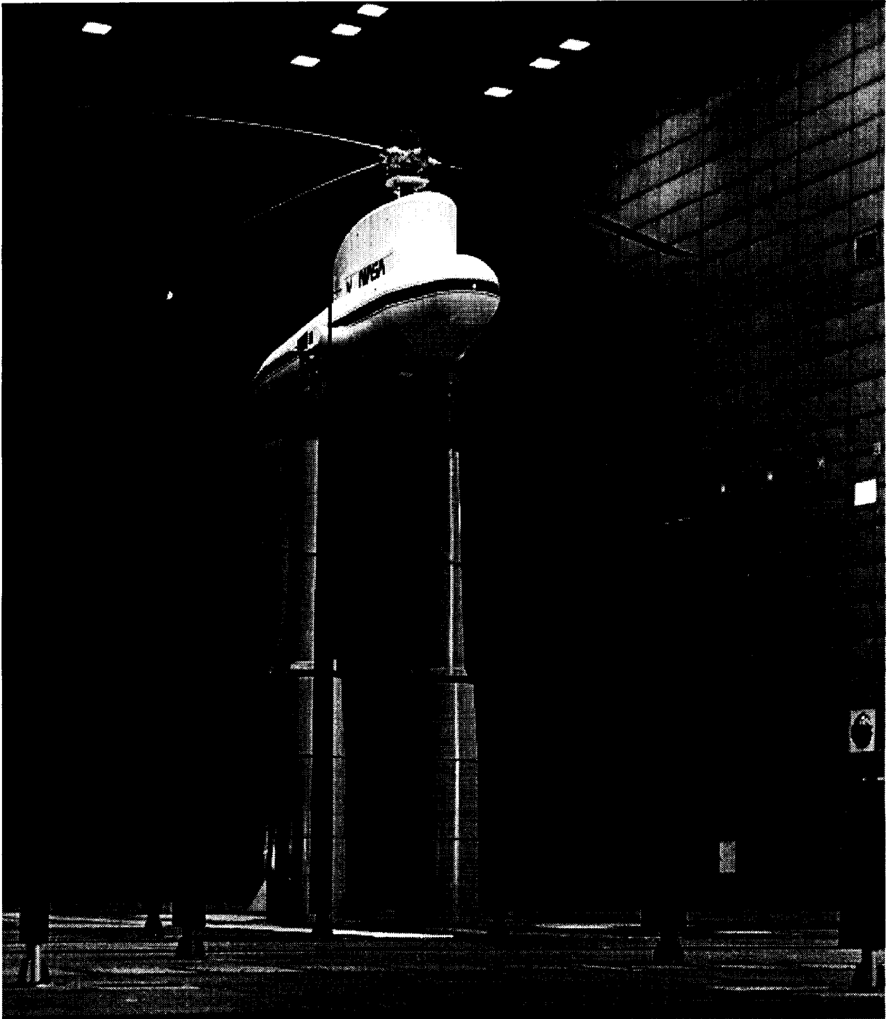
Figure 2. S-76 Rotor System installed on Rotor Test Apparatus in the Ames 80- by 120-Foot Wind Tunnel Test Section.
