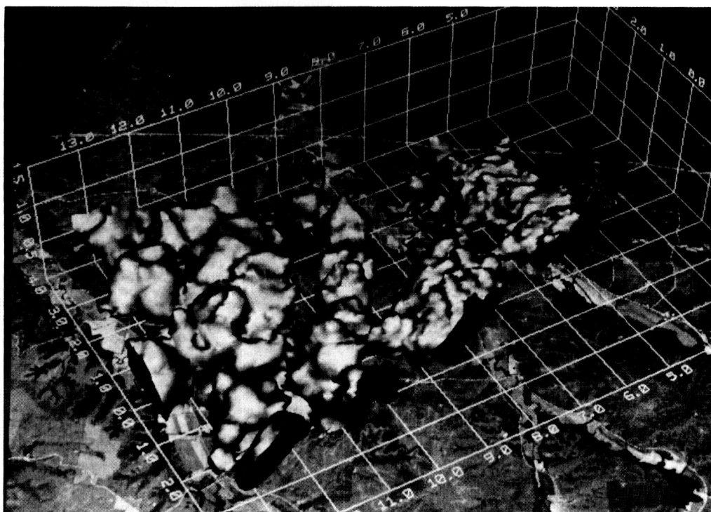
Fig. 4a. Perspective three-dimensional view of convective cells in the atmospheric boundary layer (ABL) displayed over a high-resolution SPOT picture of surface topography on July 1, 1987, at 1121 CDT under almost windless convective conditions. This display is prepared by selecting a contour layer to construct a solid surface through the volume of normalized aerosol backscatter data. The lidar is located at the origin of the coordinate system provided in the picture. All dimensions are given in kilometers. A fork-shaped creek bed area is clearly visible on the surface, with one leg at 8 km and the other one between 5 and 8 km.
