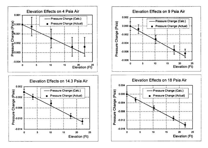
This data matches the theoretical curves to within  $\pm 0.001$  PSIA; the repeatability of our instrumentation. This error is not significant for a PSI System 8400 with 15 PSI Rackmount Modules calibrated with a 15 PSIA Digiquartz PCU.
