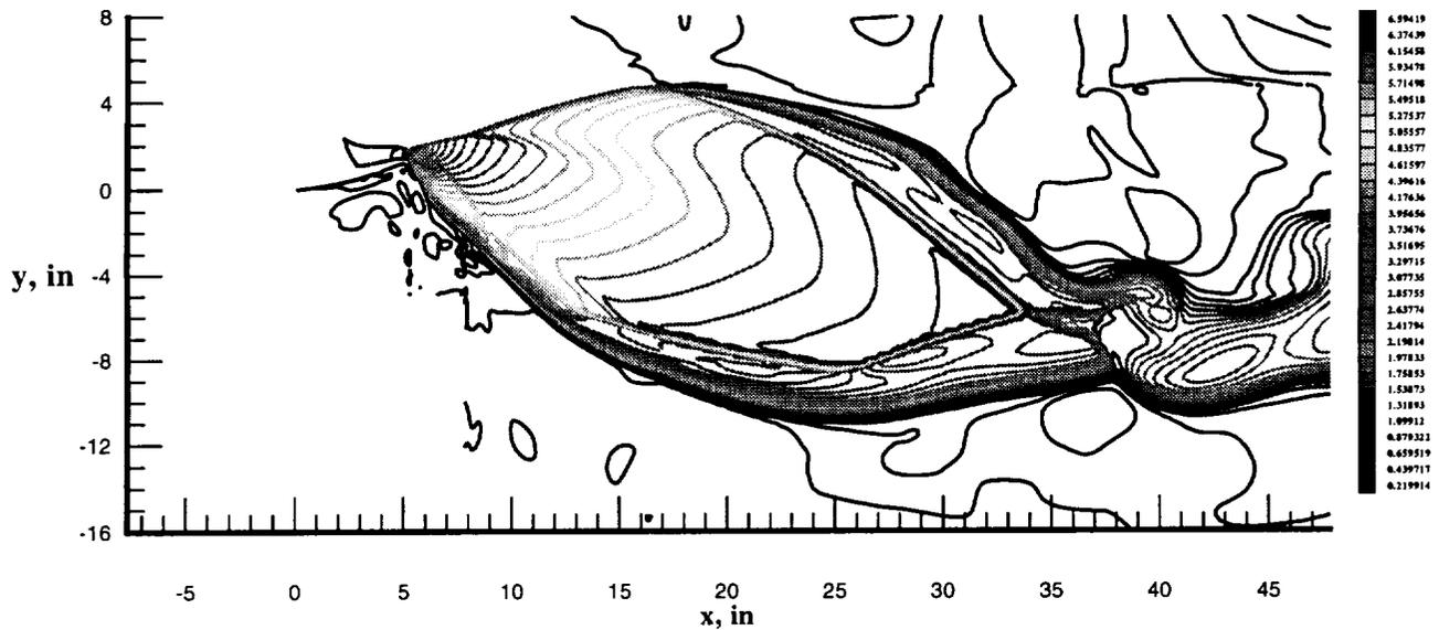
Figure 18. Predicted Mach contours along the centerline of the concave ramp, high Mach number configuration at  $M = 0.1$  and  $NPR = 102$ .
