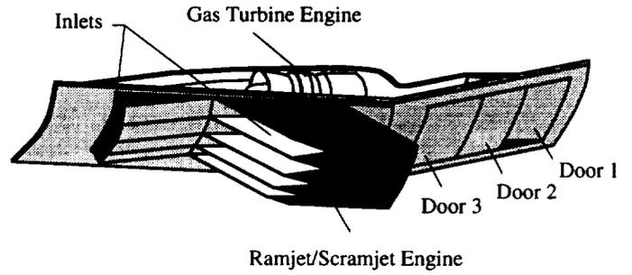
Figure 2. Translating throat single expansion-ramp nozzle integrated into the afterbody of a high-speed vehicle.
