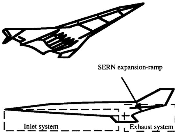
Figure 1. Sketch of a highly integrated high speed vehicle.
